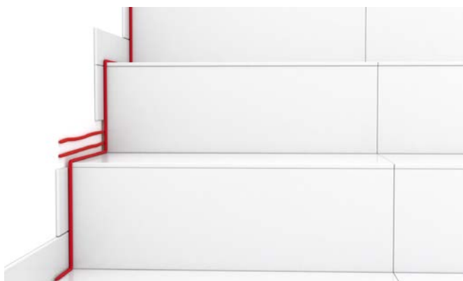
Grouting on tiles and slabs
