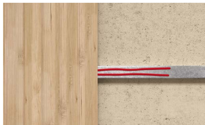
Bonding wall cladding
