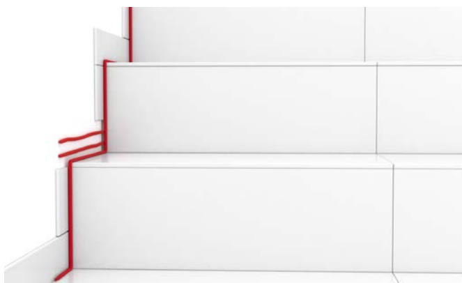
Bonding and grouting skirting boards and tiles
