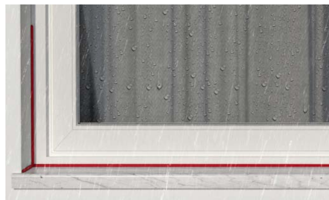
Exterior sealing joints
